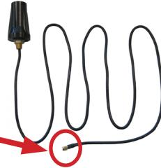
*Note: It is strongly recommended that the GPRS antenna be mounted on a horizontal plane (the top) outside the vending machine. This may be accomplished by drilling a 1/2" hole through the top of the vending machine and threading the antenna cable inside. The GPRS antenna strength may be influenced by the digital signal in the area and placement constraints in or on the vending machine.*
